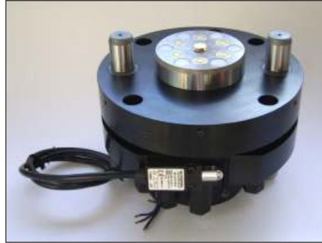
Docking station with six coupling points, pressurized coupling; in order to dock the coupling plate, it is raised by an integrated hydraulic cylinder. An electronic sensor queries the position.
