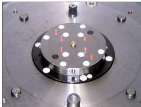
Docking system in the loading and unloading station of a machine tool. In order to allow 360° rotation of the hydraulic clamping fixture the system is equipped with a rotary coupling.
