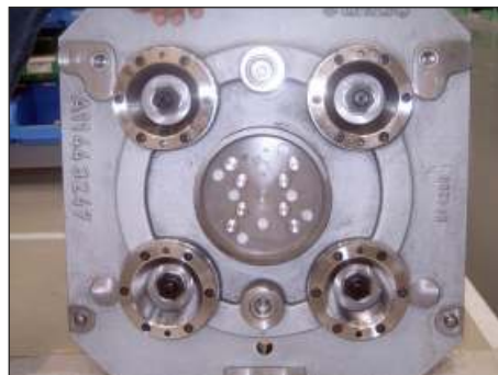
Coupling nipple plate in the fixture plate of a machine tool. The nipple plate is docked to the docking unit (figure above) and hydro-mechanically locked.
