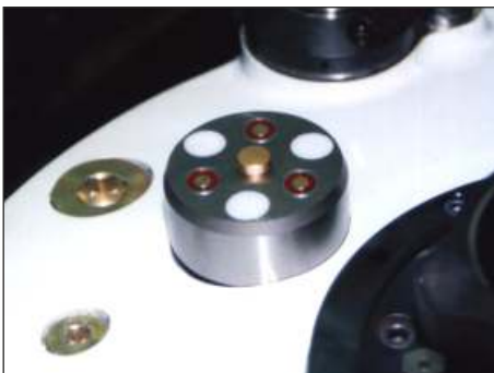
Triple coupling system for hydraulic oil fed of the fixture plate in a machine tool. The connection in the loading and unloading station is realized through the lowering of the fixture plate.
