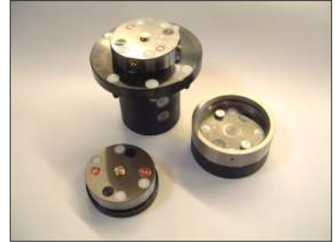
Coupling system with hydro-mechanical locking and two coupling points:
